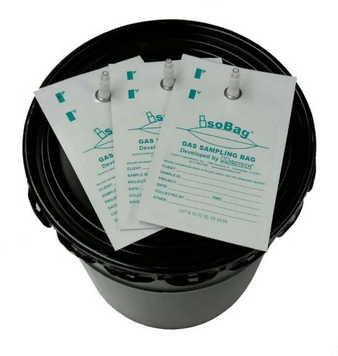
Three IsoBags<sup>®</sup> were loaded with a known gas and the concentrations were measured over three months. For most components the results show remarkable stability.
